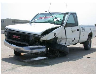
Photographs of post-test damage to vehicle used in NCHRP Report 350 crash testing of Dr. Sicking's BEAT-BP (Bridge Pier Protection System), in which Dr. Sicking and the testing facility determined that several occupant compartment deformations of greater than six inches met NCHRP Report 350 criteria.
