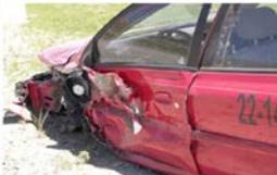
Photographs of post-test damage to vehicle used in crash testing of SKT-MSG Tangent End Terminal at Figure 37 of Report.
